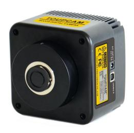
1.45M USB2.0 C-Mount Camera 2/3" Color SONY CCD Sensor SONY ICX285AQ (Progressive) Square Housing:120 X 120 X 109mm TE-Cooled System - 20 °C below Ambient Temperature Support Microsoft Windows XP / Vista / 7 /8 (32 & 64 Bit)
